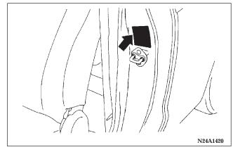
13. Check tire inflation pressure. Tire inflation pressure specifications are shown on a placard located on the driver's side "B"-Pillar.
